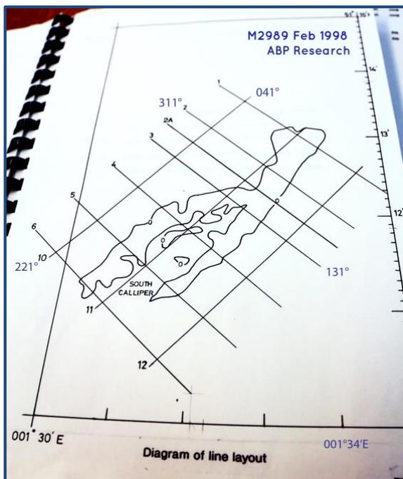
Figure 2. Grid lines from Feb 1998 survey
